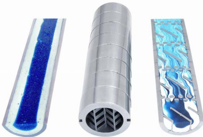
Figure #1: Mixing of blue and white epoxy resins. Empty tube (left) provides no mixing. Eight (8) GXR mixing elements (center and right) create a very high degree of mixing in a short length.
