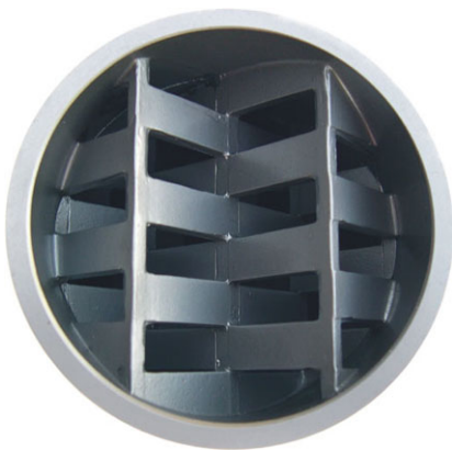
Figure #2: The GXR static mixing elements are extremely strong due to their monolithic cast construction where the mixing bars are joined to each other and to the ring wall via a single molten metal pour (metal mixing element shown above). In plastic construction, they are injection molded with the same monolithic structure.
